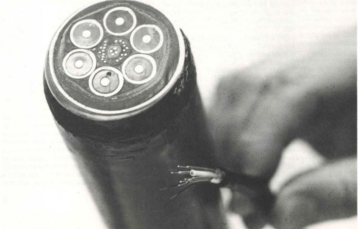
Optical fibers are rapidly replacing pair cables (above) and coaxial cables (below), thus depriving the copper industry of a vital market.
