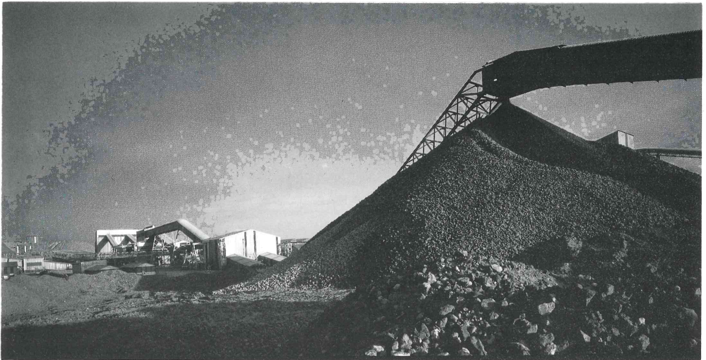
A stockpile of diamond-bearing ore at the Orapa mine, Botswana, on its way to the main treating plant.
