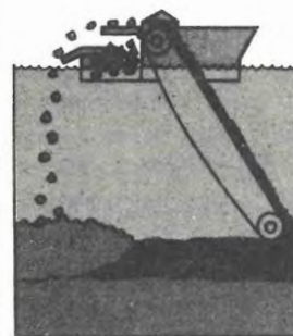
The ore is concentrated on board the dredger and waste material is dumped behind as tailings
